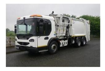
2.2.3 A new bespoke collection vehicle is also being purchased that will allow properties in remote areas to be collected using wheeled bins instead of bags, making the collection operation safer by removing an element of manual handling of bags, and be also used to support the food/recycling service where necessary. This vehicle will be a smaller size and the collection-body made of plastic that is sealed for food-waste collections.
